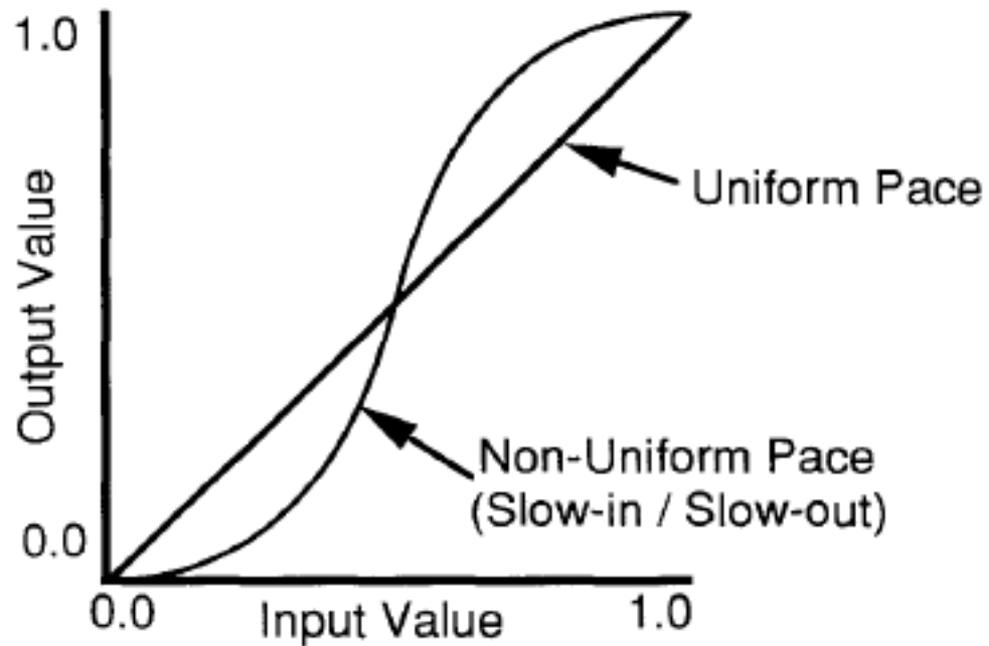
Figure 4. Two Example Pacing Functions
