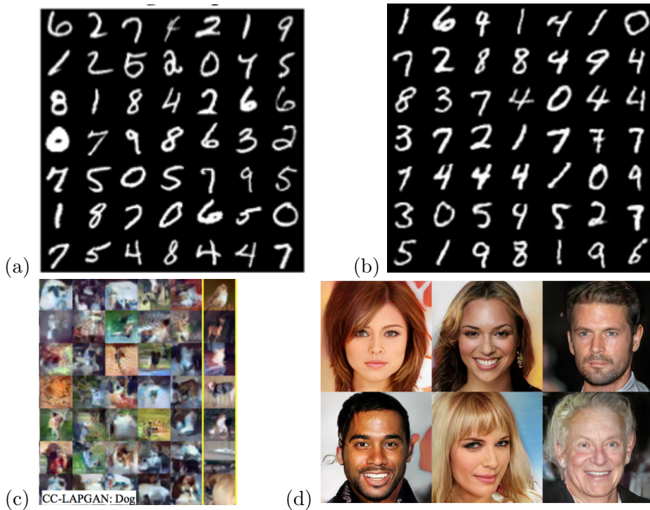
Figure 1: (a) Training images from the MNIST dataset. (b) Samples from a Deep Boltzmann Machine (Salakhutdinov and Hinton, 2009). (c) Samples from a GAN trained on the “dog” category of CIFAR-10 (Denton et al., 2015) (d) Samples from a GAN trained on images of celebrities (Karras et al., 2017).
